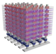
Three-dimensional resistive switching cross-bar array memories are highly desirable future memory devices for data centric computation. Issues in the circuitry, integration, and material properties of the two- and three-dimensional crossbar array memories are dealt with in a quantitative manner. The impressive progress in theoretical understanding and fabrication of these devices achieved during the past decade is summarized, and an outlook on possible applications is further provided.
