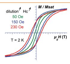
The interplay between dipolar interaction, surface anisotropy, and size control at the molecular level allows the fine tuning of the magnetic anisotropy, the energy barrier for the reorientation of the magnetization, and the blocking temperatures (4 to 22 K) of individual CsNiCr(CN)<sub>6</sub> coordination nanoparticles. Upon dilution of the objects, the coercive field shifts from 50 to 230 Oe for 6 nm objects, highlighting the contribution of surface anisotropy.
