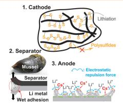
The highest areal energy density to date of a lithium-sulfur battery is demonstrated by the combined smart engineering of the key cell components (electrode, electrolyte, and separator). The integrated strategy suppresses both lithium polysulfide dissolution from the sulfur cathode and lithium dendrite growth from the lithium anode, leading to the highest areal capacity of 9 mAh cm<sup>-2</sup> while preserving stable cyclability.
