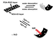
Near-infrared (NIR) light-driven bilayer actuators are fabricated by exploiting the photothermal conversion and humidity-sensitive properties of polydopamine-modified reduced graphene oxide. The bilayer actuator is capable of fast, highly efficient, and reversible bending/unbending motions toward periodic NIR light irradiation. The bilayer actuator is also utilized to build a NIR light-driven walking device capable of performing quick worm-like motion.
